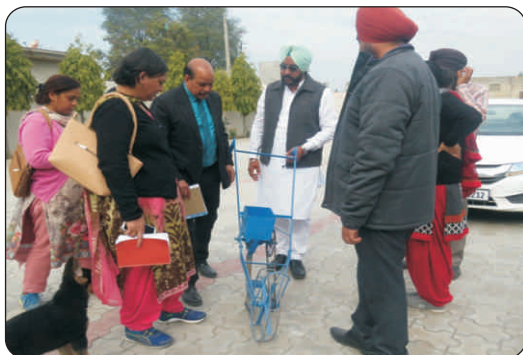
Fig 16: Manually operated single row seed drill for rapeseed-mustard developed by PAU Ludhiana and used in CFLDs
